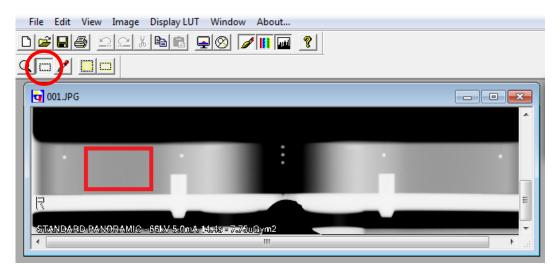
5. Check the window "Statistics": the S\N (db) value has to be higher than 25.
