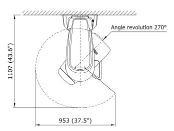
Figure 3: I-MAX dimensions Wall mounted version
