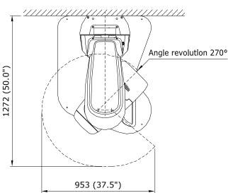
Figure 5: I-MAX dimensions Floor mounted version
