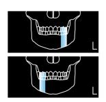
The bitewing mode, right or left, means that only the corresponding dentition sector is irradiated; the emission will start from the beginning, to just after the mid sagittal plane for the right part. For the left, it will start just before the mid sagittal plane and continue until the end of the rotation. The exam is performed with the same trajectory of the ortho rad panoramic exam, reducing the rays' emission time to include just molar and pre-molar teeth.
