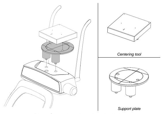
Figure 6: Support plate and centering tool positioning
